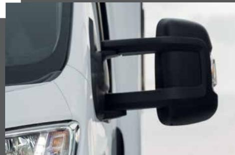
Electrically heated and adjustable wing mirrors with blind-spot mirror
