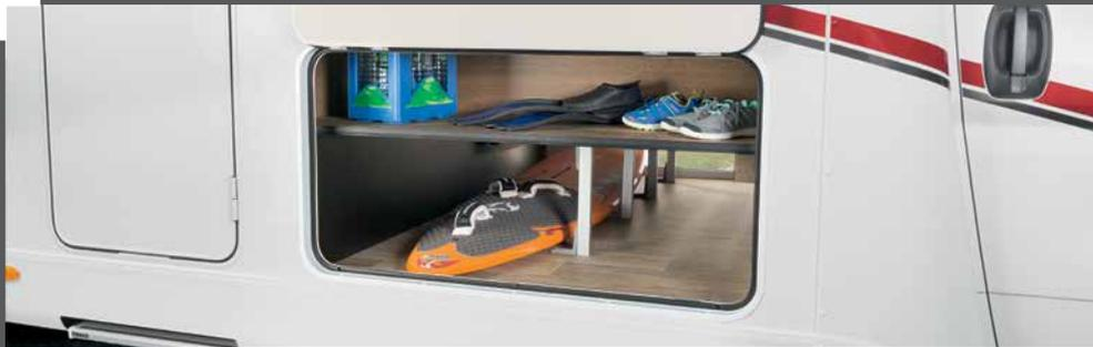
The A 7877-2 model is winterproof thanks to the raised double floor, which can be partially loaded across the entire width of the vehicle. The complete water system is housed in this heated underfloor compartment and thus protected from frost
